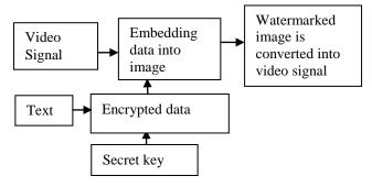
Fig.1 Block diagram of data embedding using watermarking
